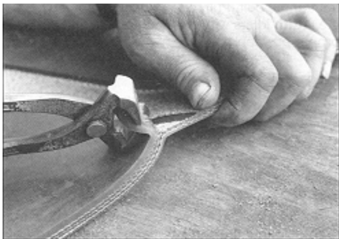
Figure 6 Carpenter's claw-type pincers are used for pulling away sections of belt cover and fabric plies.
