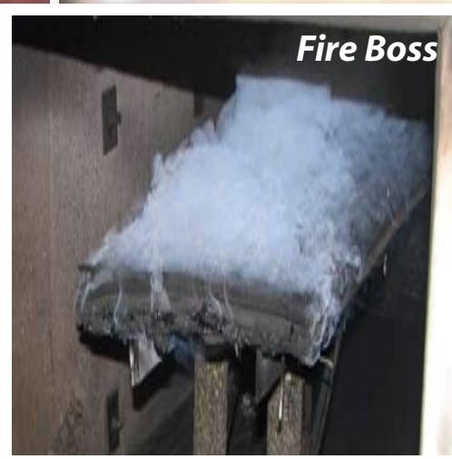
Belt condition one minute after 5 minute test burn time.
